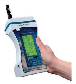
The YESAIR is a battery powered, portable air quality detection and data logging instrument designed for intermittent or continuous indoor air quality monitoring.
