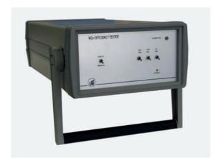
In order to valid NOx measurements, the efficiency of the NO2 converter must be higher than 90 %, it is therefore very important to check easily and precisely the efficiency of the NO2 converter.
